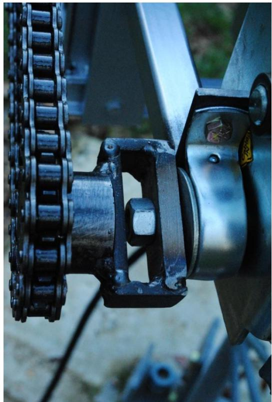
The sprockets used in this project are available at Tractor Supply or similar hardware store. They are designed to be used in a keyed configuration or suitable for welding as illustrated to the left. Unfortunately the winch shaft is not "keyed" in a manner accommodating these sprockets.
