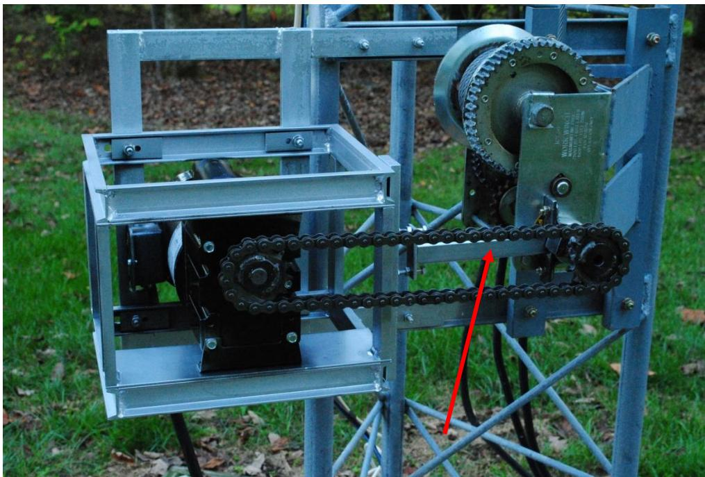
The picture to the left reveals further details of the construction. Of particular note is the steel member between the winch axle thrust bearing and the attachment to the right side of the gear motor cage. This is identified by the red arrow in the figure. This member greatly restricts any oscillatory movement to the left and right between the gear motor and the winch. It is *mandatory* or the chain may "eat itself". Without
