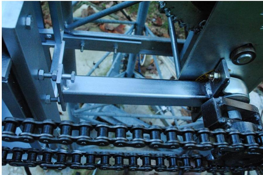
To the left is a close-up of this important restraining member. The left side is somewhat floating, with force in +/- x directions being provided by the positions of the nuts on the two grade 8 bolts. If detached on the left, the assembly will just free-rotate on the winch shaft bearing to a vertical position. All the force is in the +/- x directions, provided everything is lined up ☺.
