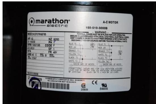
One can readily see that the motor is  $\frac{1}{2}$  HP and careful attention must be paid to its wiring. The motor is controlled by a phase reversal switch (~ \$75) which must be properly wired or you will not have favorable results. The details of the wiring are on the "Marathon Electric" faceplate above. While this gear motor is suitable for mounting outdoors, I plan to place some type of "roof" over the assembly to afford some additional protection from the elements.
