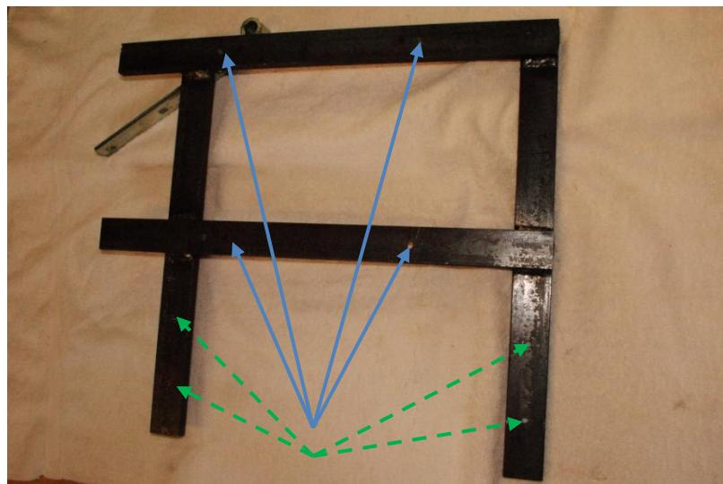
Mounting to the tower is accomplished with the assembly to the left. Each member is 2" x 1/2" steel plate. The blue arrows (solid lines) identify the holes used to attach the cage assembly just discussed. The green dotted lines are the holes used to attach to the tower.
