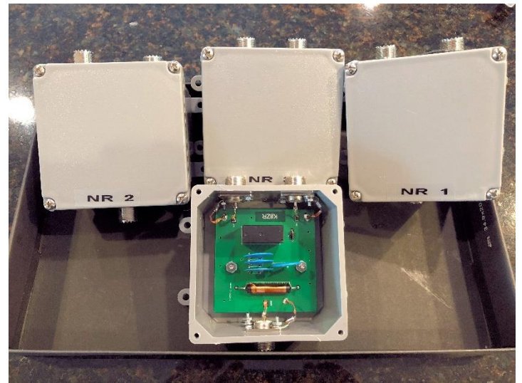
Figure 12 Four Remote RF Switch Units
