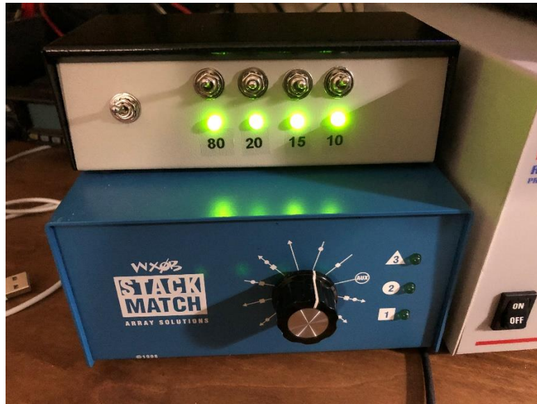
Figure 14 Controller Activating All Four Alternate Antennas
