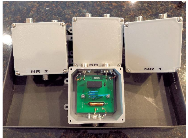
Figure 12 Four Remote RF Switch Units
